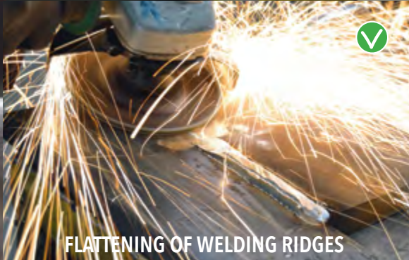
FLAT GRINDING WITH AN ANGLE BETWEEN 10-15°
